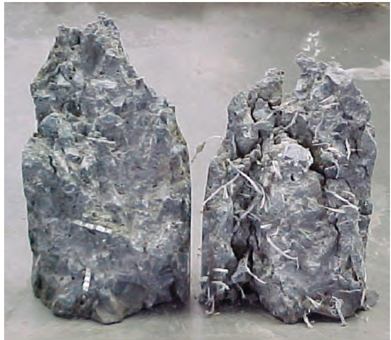
Left: Steel fibers at 40 lbs/yd results in a low fiber count. Right: STRUX 90/40 at only 4.5 lbs/yd produces a high fiber count and improved plastic shrinkage cracking control.
